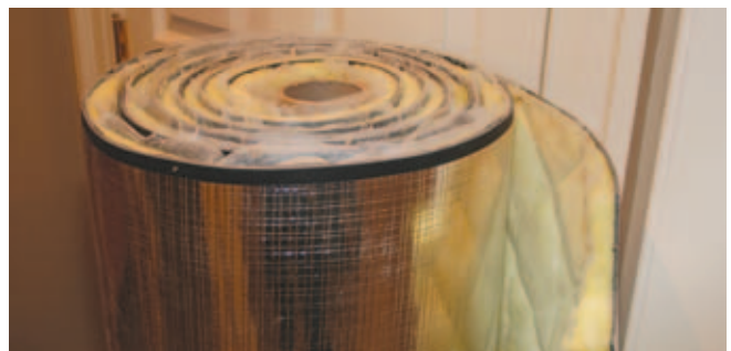
Figure 6. All piping — including water-supply and waste lines, gas lines, and electrical conduits — should be wrapped (above) and the joints sealed with silicone (above right). The author prefers special fiberglass acoustic pipe insulation with a layer of mass-loaded vinyl inside (right). The insulation prevents noise from traveling between rooms via pipes and minimizes the sound of running water.
