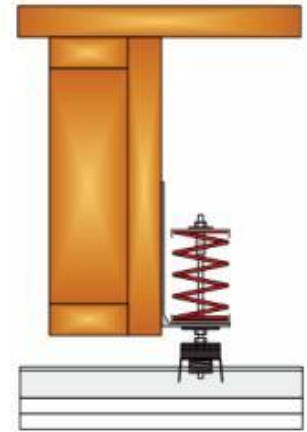
RSIC-1-SI INSTALLATION WITH FRAMING SPACED @ 16” OC. & RSIC-1-SI @ 24” OC.
